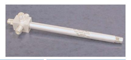
Microlab Model Dx-88FN series of 2, 3 and 4 way Power Splitters has been designed to evenly split high power cellular signals with minimal reflections or loss. All joints are moisture sealed to meet the IP67 rating. The mechanical shape allows simple attachment to wall using the supplied clip and bracket.
