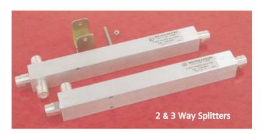
Microlab Model Dx-51/55FN series of 2, 3 and 4 way Power Splitters has been designed to evenly split high power cellular signals with minimal reflections or loss. The wide frequency range allows use with multiband antennas and leaky cable systems.
