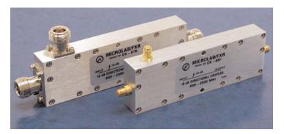
Microlab CK-60 series of N and SMA Directional Couplers, is a two section, quarter wave, air-line design for indoor applications covering all wireless bands to 2,500 MHz. Units couple off a defined fraction of signal from 5 to 30 dB with minimal reflections or loss.
